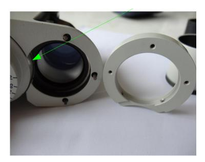
Right holder is keep as is. Eyepiece holder will be glued on it
