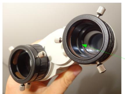
Due to the gap, there are tiny/faint stray lights in the right holder that could be anoying when looking at the sun in H-Alpha.
