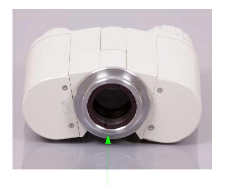
The default head is the same than the one of the MarkV. With Zeiss Bajonet and M34 female Thread for Glass path. No work is mandatory.
